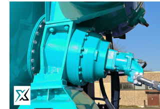
Gearbox, pump & motor from ZF, PMP, Bosch Rexroth
